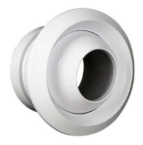
**Description** The LinkedAir jet nozzle diffusers are designed for supply air application that requires a long throw with high air velocity, supply large amount of conditioned air into one space. They can be easily adjusted to any throw direction with 360° rotation. They can easily mount to the round ducts, and they have low pressure losses and low noise levels.
